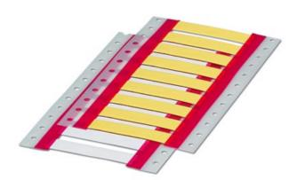
Marker for thermal transfer printer, perforated 1-way, white, labeling field:  $50 \times 16$  mm, can be used for 9.5 mm diameter, shrinkage ratio 3:1, 1 roll = 500 Marker at 50 mm
